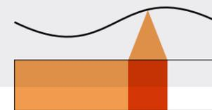
**Spotlight** - Radar continuously images or monitors a preselected area of ground as the aircraft flies past or around it.
